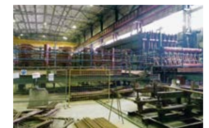
Assembly of a heating surface unit of the convection shaft and a platen superheater unit
